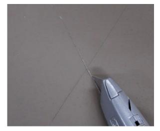
**3.** Tape is applied over the center of the cuts and pressed firmly to ensure good contact. A portion on the end of the tape is left loose in order to pull.
