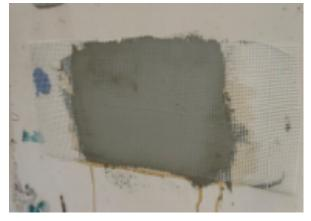
**5.** Once the test material has cured/dried, take the loose end of mesh or fabric and pull it straight out from the wall surface.
