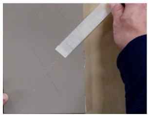
5. Compare the resulting amount of coating that is left intact to the levels included in ASTM D3359 for a rating.
