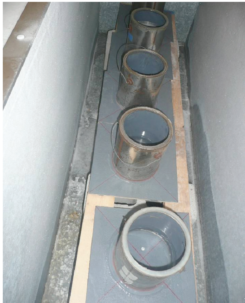
ASTM D1970 test apparatus. This test measures the ability of a barrier material to self-seal around two nails in a manner sufficient to prevent a column of water from seeping through the penetration.
