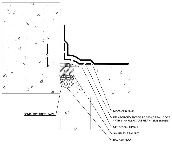
NOTES: REFER TO SYSTEM GUIDE FOR PRIMING, SIKAGARD 7600 THICKNESS, PROTECTION BOARD, AND DRAINAGE MAT **REQUIREMENTS**
