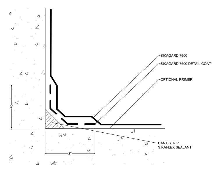
NOTES: REFER TO SYSTEM GUIDE FOR PRIMING, SIKAGARD 7600 THICKNESS REQUIREMENTS
