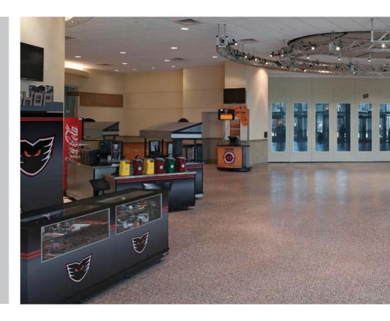
morning the Bazella Group scraped off the excess flakes for reuse, and cleaned and vacuumed the floor. A topcoat was then applied to give the floor a glossy appearance, and left to cure for six to eight hours.
