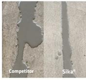
**THICKER BODY** Won't run out after placed in a joint but holds a nice ridge. Less staining.
