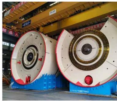
TUNNEL BORING MACHINES (TBMs) are commonly found with diameters from 5 to 17 meters and increasing. There are also the micro TBMs which are smaller, have an excavation diameter up to 4 meters and are extensively used today to construct kilometres of underground infrastructure worldwide.
