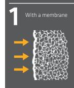
With a membrane The **FILTER CAKE** membrane forms a thin impermeable layer directly on the wall, transforming excess slurry ressure into effective support stress in low permeability grounds. The slurry creates only a surface impermeabilization, typically several mil-
