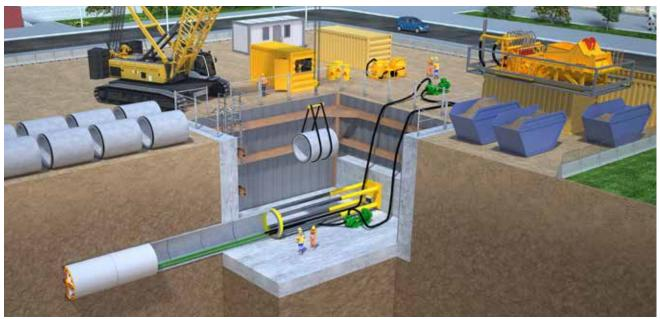
Microtunneling is a fast alternative to conventional pipe installation systems. It is a fully automated method of boring and pipe installation without the need for disturbing the surface. Micro TBMs start at diameters from a few centimetres and increase up to 4 meters. They are typically used for excavation of many of the vital utility facilities such as fresh water, wastewater, oil, gas, communications and electricity.
