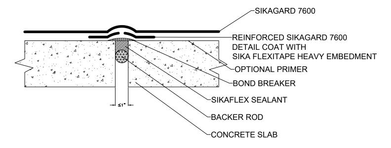
NOTES: REFER TO SYSTEM GUIDE FOR PRIMING, SIKAGARD 7600 THICKNESS, PROTECTION BOARD, AND DRAINAGE MAT REQUIREMENTS
