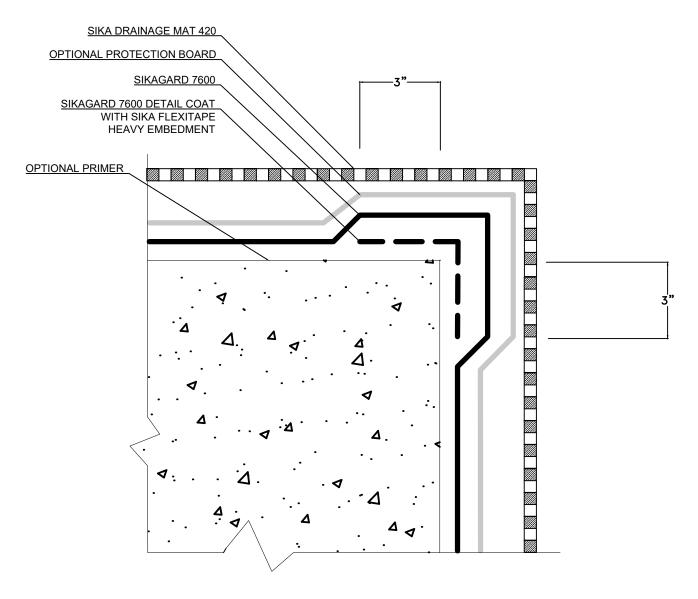
NOTES: REFER TO SYSTEM GUIDE FOR PRIMING, SIKAGARD 7600 THICKNESS, PROTECTION BOARD, AND DRAINAGE MAT REQUIREMENTS
