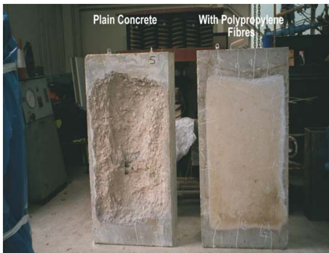
Figure 2. Test samples from CTRL testing - plain concrete & concrete with PP fibres.
