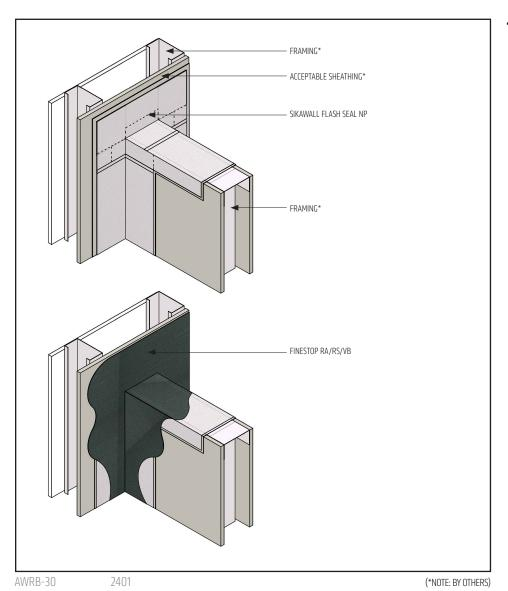
Fully coat SikaWall Flash Seal NP with Finestop RA/RS/VB.
