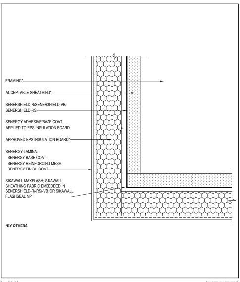
Ensure Flexguard 4, SikaWall Intermediate 6 or SikaWall Intermediate 12 Reinforcing Mesh is lapped a minimum of 8" (203 mm) around corners.
