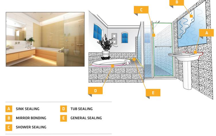
A / C / D / E Sikasil® N-Plus - is a general purpose, one-component, non-sag, elastomeric, 100% RTV neutral cure silicone sealant. Meets the requirements of ASTM C-920, Type S, Grade NS, Class 25, Use NT, T, M, G, A, O; TT-S-00230C, Type II, Class A; TT-S-001543A, Class A; CAN/CGSB-19.13-M87, AAMA 802.3 Type II, AAMA 803.3, AAMA 805.2, AAMA 808.3. Fungicide additive for mildew resistance
