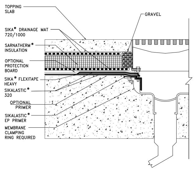
NOTES: REFER TO SYSTEM GUIDE FOR PRIMING, SIKALASTIC 320 THICKNESS, PROTECTION BOARD, AND DRAINAGE MAT REQUIREMENTS
