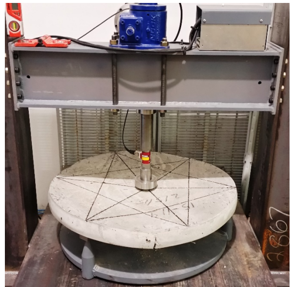
Figure 6 | ASTM C1550 Shotcrete Round Panel Test
