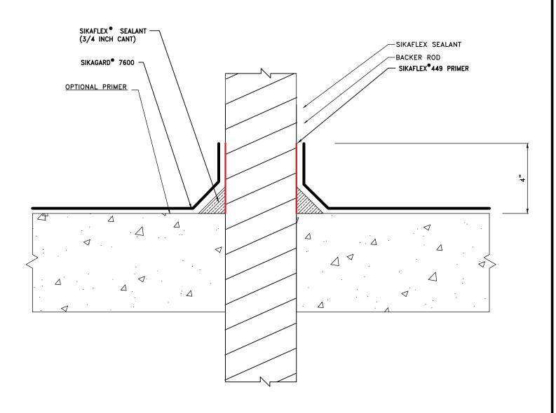
NOTES: REFER TO SYSTEM GUIDE FOR PRIMING, SIKAGARD 7600 THICKNESS REQUIREMENTS
