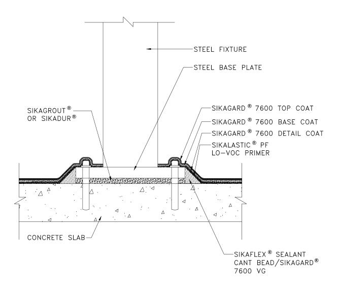
NOTES: REFER TO SYSTEM GUIDE FOR PRIMING, SIKAGARD 7600 THICKNESS REQUIREMENTS
