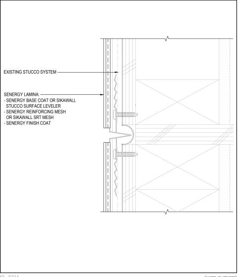
Ensure expansion joints are honored and reinforcing mesh and base coat is not continuous over the joint.
