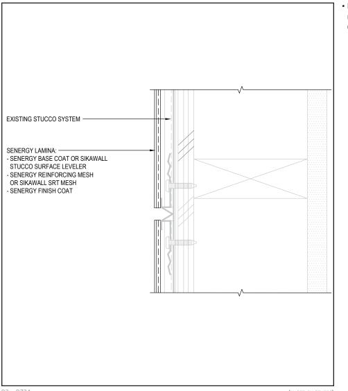
• Ensure control joints are honored and reinforcing mesh and base coat is not continuous over the joint.
