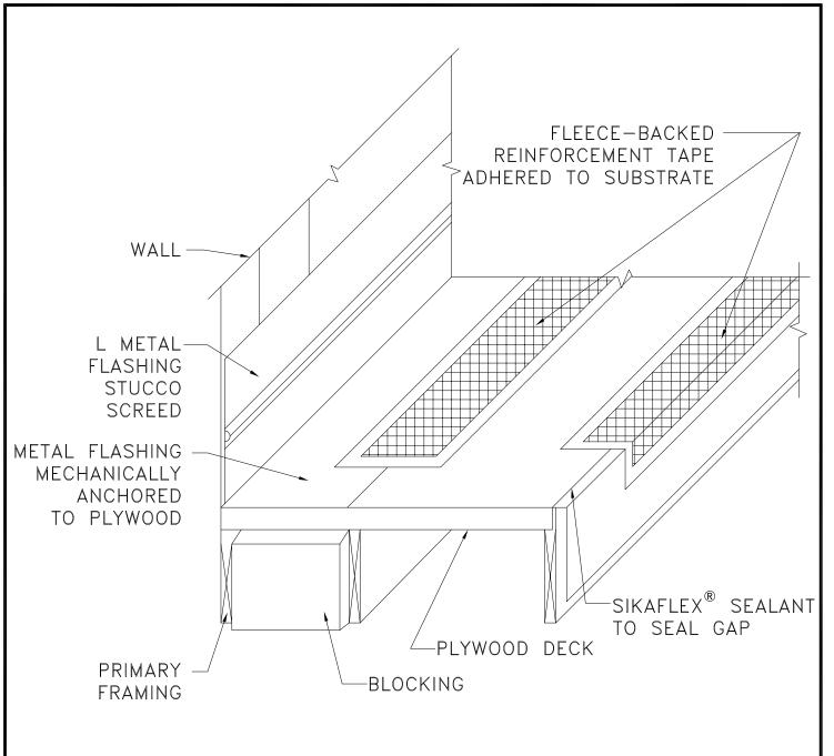
NOTE: SIKALASTIC  $^{\circledR}$  MEMBRANE NOT SHOWN FOR CLARITY. MEMBRANE TO BE INSTALLED ON PLYWOOD DECK AND METAL FLASHING. TERMINATE DECK COATING AT FACE OF WALL.
