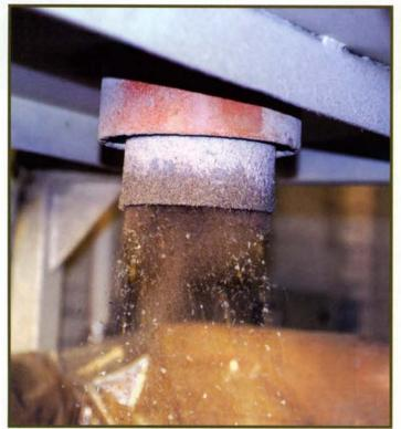
Figure 7 - PVC membrane being ground for recucling.
