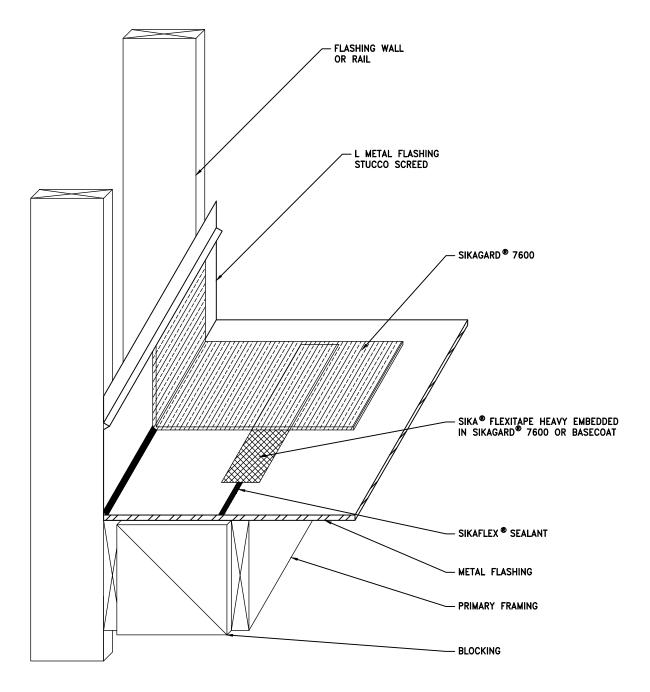
NOTES: REFER TO SYSTEM GUIDE FOR PRIMING, SIKAGARD 7600 THICKNESS, PROTECTION BOARD, AND DRAINAGE MAT REQUIREMENTS
