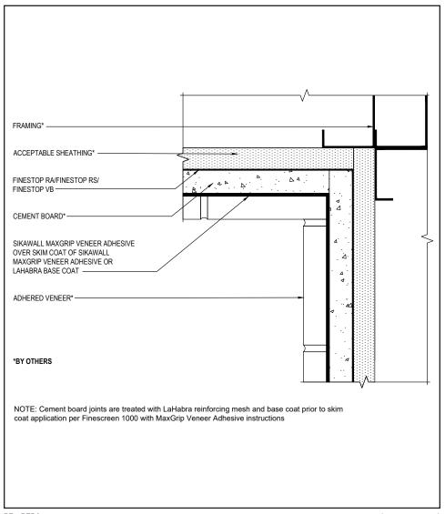
Cement board sheathing joints must be treated with LaHabra reinforcing mesh and base coat prior to skim coat application of SikaWall MaxGrip Veneer Adhesive.
