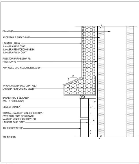
Ensure EIFS termination is fully encapsulated with mesh reinforced base coat. Pre-backwrap both the vertical and horizontal terminations. Extend reinforcing mesh a minimum of 2½" onto back of insulation board.
