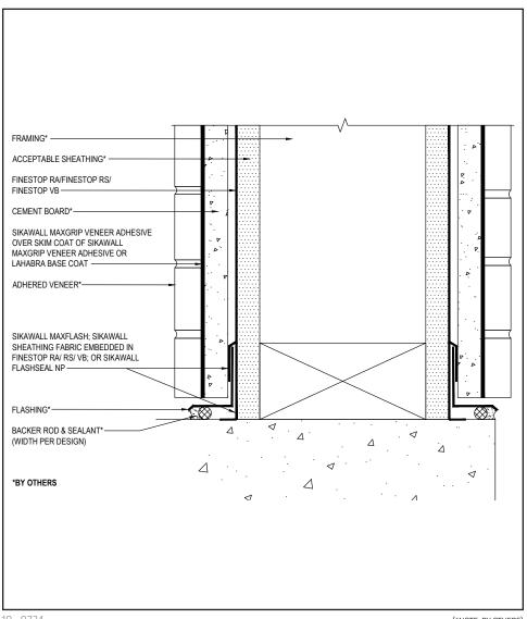
Terminate the Finescreen 1000 CI with MaxGrip system a minimum of 4" (101 mm) above raw earth and 1" (25 mm) above paved surface.
