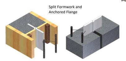
Waterstop Should Be Aligned With The Center Of The Joint. Size And Style Of The Waterstop Determine Permissible Variation From The Centerline. Contact Sika (St. Louis Sales Office) For Specific Guidelines.
