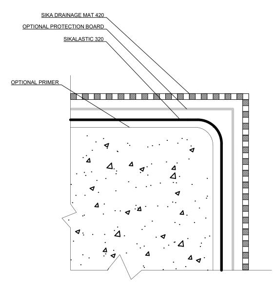
NOTES: REFER TO SYSTEM GUIDE FOR PRIMING, SIKALASTIC 320 THICKNESS, PROTECTION BOARD, AND DRAINAGE MAT REQUIREMENTS
