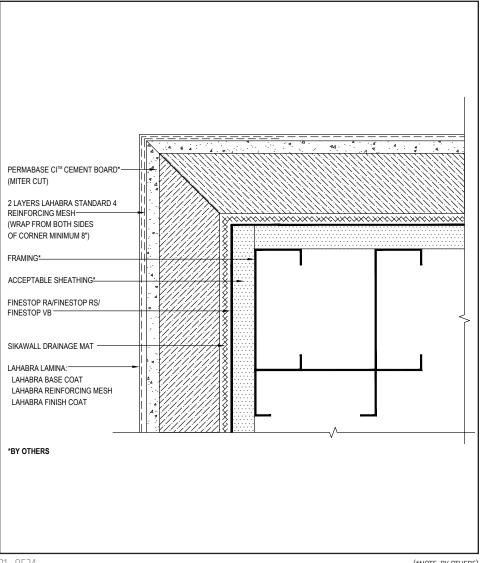
Ensure Standard Reinforcing Mesh is lapped a minimum of 8" (203 mm) around corner on both sides.
