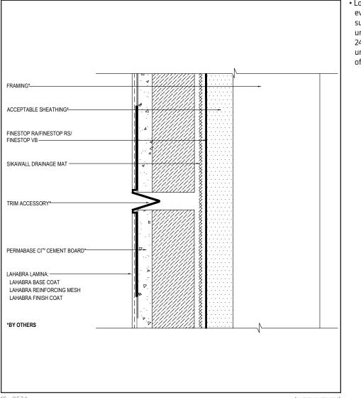
· Locate control joints approximately every 600 ft.2 (56 m2) of wall surface area with maximum uncontrolled length or width of 24 lin. ft. (7 m) and a maximum uncontrolled length-to-width ratio of 2 ½:1.
