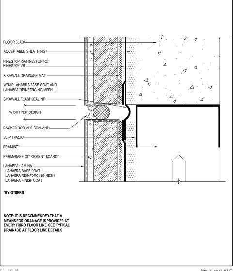
termination with mesh reinforced base coat. Extend reinforcing mesh a minimum of 2 ½" onto back of insulation board.
