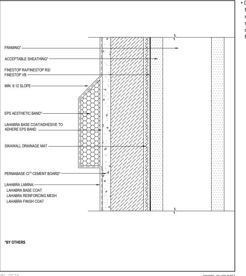
On horizontal projections greater than 1" (25mm) maintain a minimum 6:12 slope. For sloped surfaces over 24" (340mm), a roofing system or a metal cap flashing is required.
