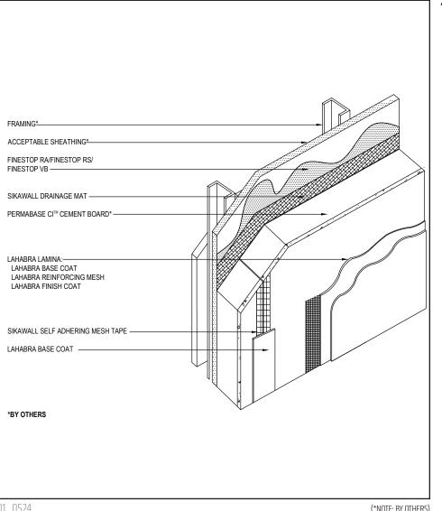
• Install PermaBase CI composite cement board panel over LaHabra air/water-resistive barrier and SikaWall Drainage Mat per manufacturers' recommendations, applicable building code and project requirements.
