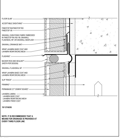
Fully encapsulate system termination with mesh reinforced base coat. Extend reinforcing mesh a minimum of 2 <sup>1</sup>/<sub>2</sub>" onto back of insulation board.
