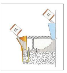
Schematic of side view of grout flow through a head box.\*
