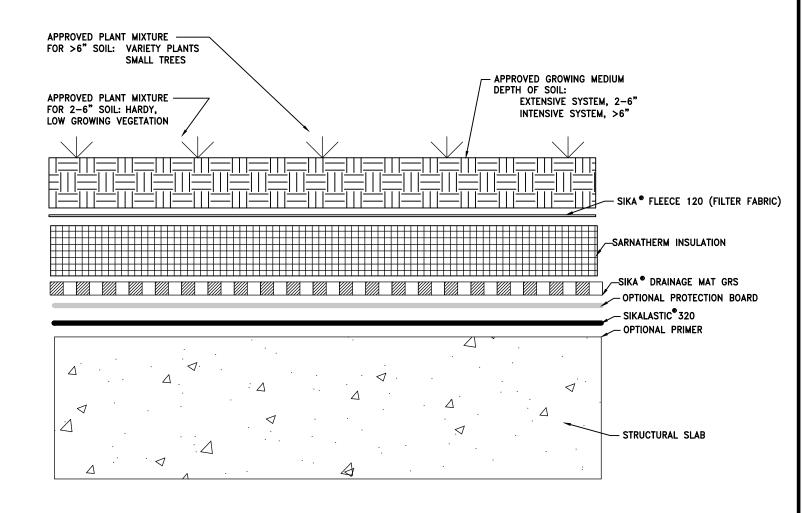
NOTES: REFER TO SYSTEM GUIDE FOR PRIMING, SIKALASTIC 320 THICKNESS, PROTECTION BOARD, AND DRAINAGE MAT REQUIREMENTS
