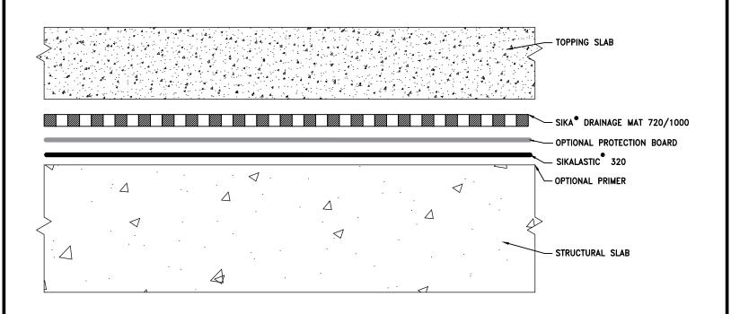
NOTES: REFER TO SYSTEM GUIDE FOR PRIMING, SIKALASTIC 320 THICKNESS, PROTECTION BOARD, AND DRAINAGE MAT REQUIREMENTS
