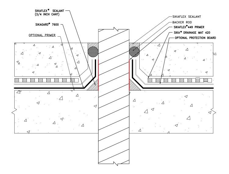
NOTES: REFER TO SYSTEM GUIDE FOR PRIMING, SIKAGARD 7600 THICKNESS, PROTECTION BOARD, AND DRAINAGE MAT REQUIREMENTS
