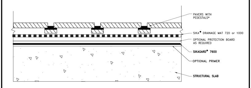
NOTES: REFER TO SYSTEM GUIDE FOR PRIMING, SIKAGARD 7600 THICKNESS, PROTECTION BOARD, AND DRAINAGE MAT REQUIREMENTS
