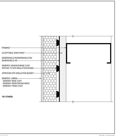
• All terminations must be fully encapsulated with mesh reinforced base coat. Prebackwrapping is recommended at drainage terminations. Extend reinforcing mesh a minimum of
