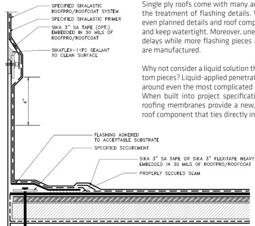
Single ply roofs come with many advantages however one short coming is the treatment of flashing details. When new single ply roofs are installed even planned details and roof components can be difficult to properly flash and keep watertight. Moreover, unexpected details can arise causing project delays while more flashing pieces are delivered or while custom flashings are manufactured.
