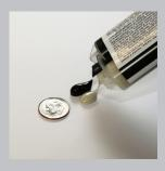
Purge dime-sized amount of material to level plungers before attaching static mixer.
