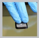
7 Bond part to glass or vehicle body within open time (50 seconds at 73°F)¹. Compress the adhesive to 0.5 – 1.0 mm (0.02" – 0.04") and scrape away any excess material. Tape can be applied, but is not required for most applications.
