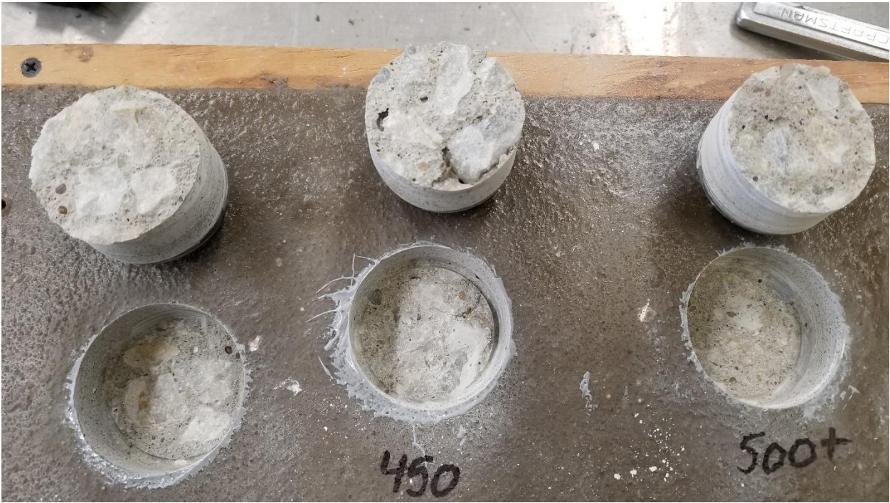
Figure 2: Sample after bond testing. In all cases, the failure occurred within the concrete substrate.
