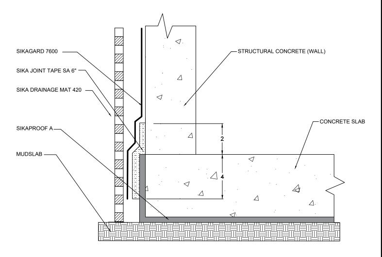
NOTES: REFER TO SYSTEM GUIDE FOR PRIMING, SIKAGARD 7600 THICKNESS AND DRAINAGE MAT REQUIREMENTS
