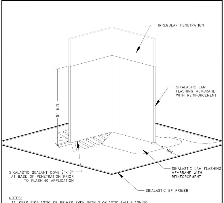
1) KEEP SIKALASTIC EP PRIMER EVEN WITH SIKALASTIC LAM FLASHING.
