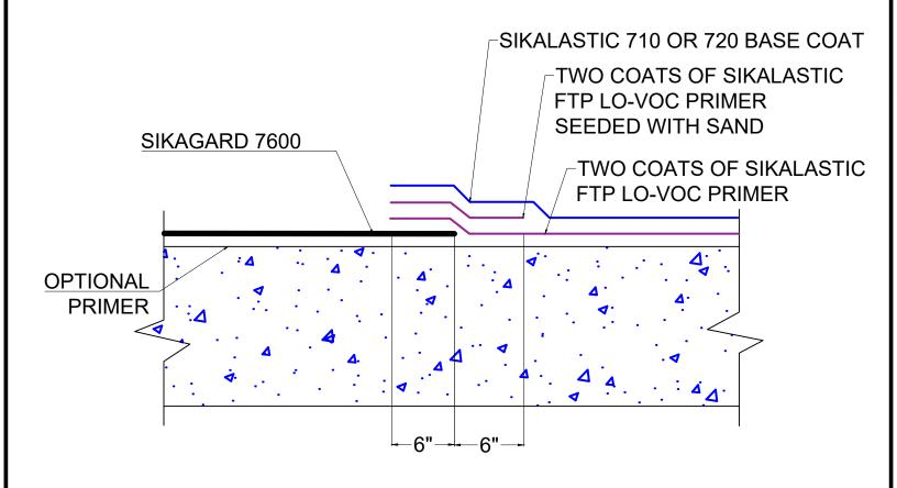
NOTES: REFER TO SYSTEM GUIDE FOR PRIMING, SIKAGARD 7600 THICKNESS, PROTECTION BOARD, AND DRAINAGE MAT REQUIREMENTS
