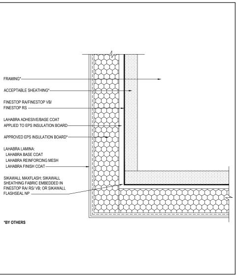
Ensure Standard, SikaWall Intermediate 6 or SikaWall Intermediate 12 Reinforcing Mesh is lapped a minimum of 8" (203 mm) around corners.
