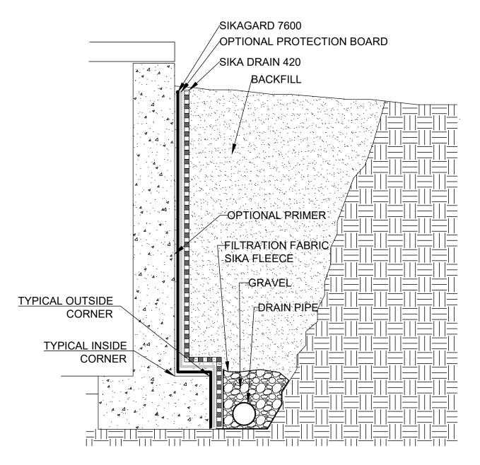
NOTES: REFER TO SYSTEM GUIDE FOR PRIMING, SIKAGARD 7600 THICKNESS, PROTECTION BOARD, AND DRAINAGE MAT REQUIREMENTS
