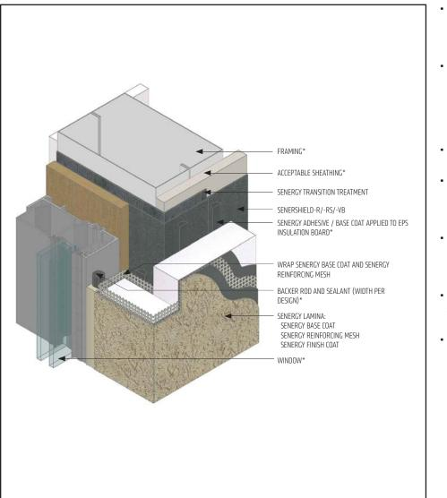
All terminations must be fully encapsulated with mesh reinforced base coat. Extend reinforcing mesh a minimum of 2 1/2" onto back of insulation board.
