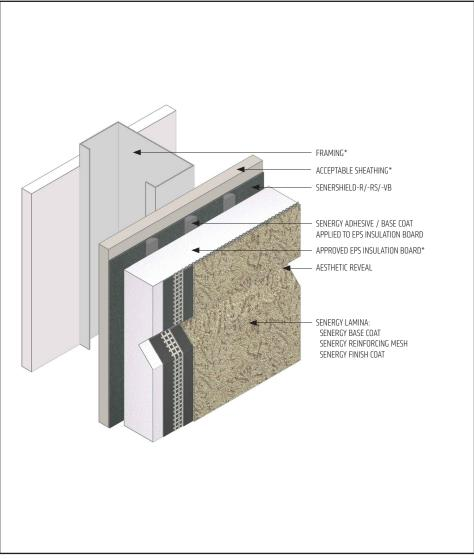
Maintain a continuous layer of EPS insulation board, at a minimum 3/4" (19 mm) thickness, behind all reveals and aesthetic grooves.
