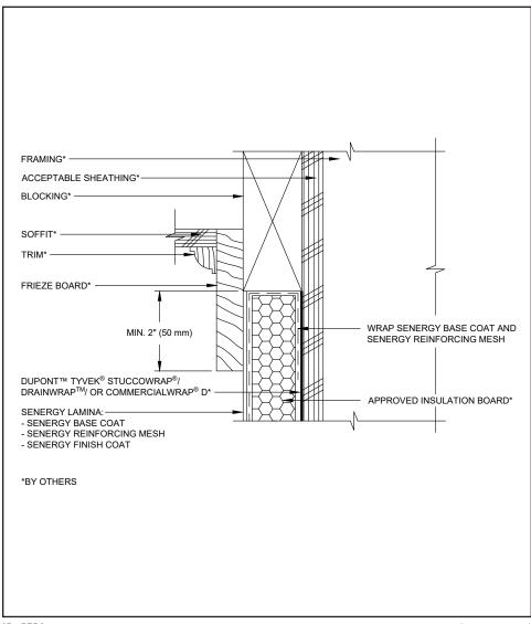
All terminations must be fully encapsulated with mesh reinforced base coat. Extend reinforcing mesh a minimum of 2 ½" onto back of insulation board.
