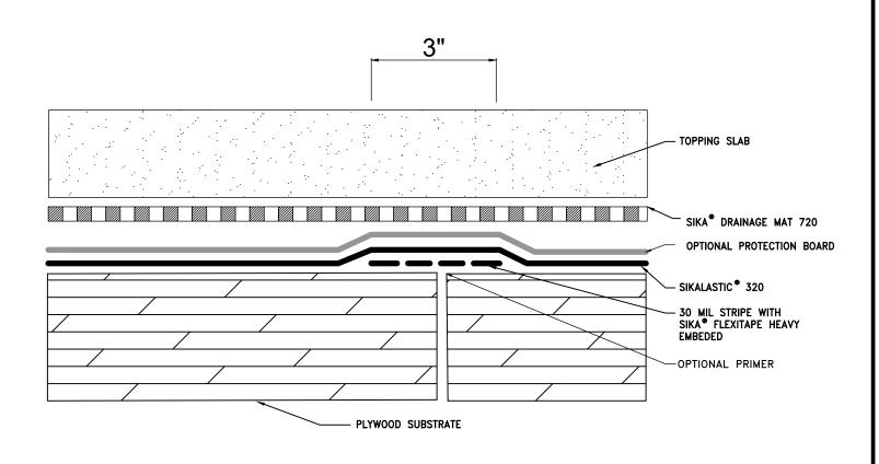
NOTES: REFER TO SYSTEM GUIDE FOR PRIMING, SIKALASTIC 320 THICKNESS, PROTECTION BOARD, AND DRAINAGE MAT REQUIREMENTS
