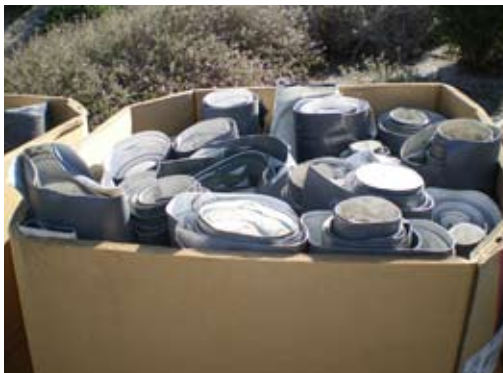
Older vinyl roofing in Sika Sarnafil-supplied Gaylords for shipment to a recycling center.
