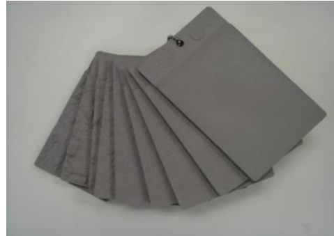
Prepared surface profile stretched flat to show comparative actual surface available for bonding
