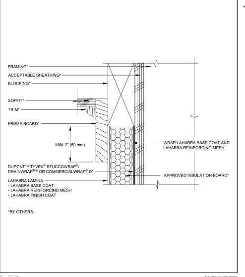
All terminations must be fully encapsulated with mesh reinforced base coat. Extend reinforcing mesh a minimum of 2 <sup>1</sup>/<sub>2</sub>" onto back of insulation board.
