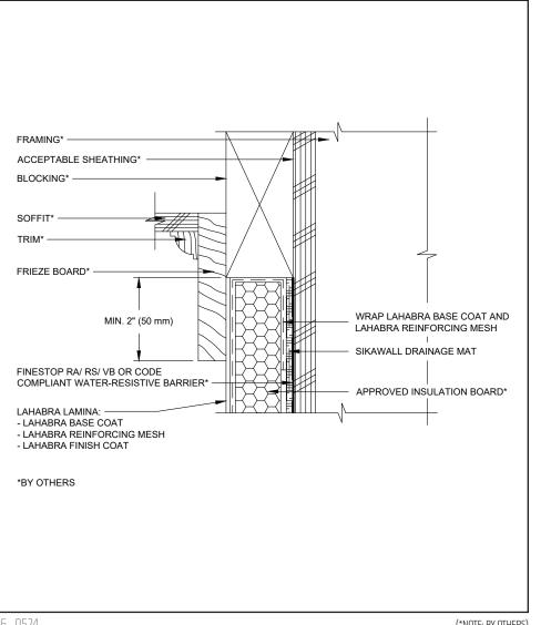
• All terminations must be fully encapsulated with mesh reinforced base coat. Extend reinforcing mesh a minimum of 2 1/2" onto back of insulation board.
