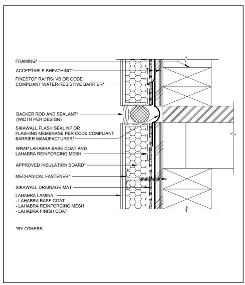
All terminations must be fully encapsulated with mesh reinforced base coat. Pre-backwrapping is recommended at drainage terminations. Extend reinforcing mesh a minimum of 2 1/2" onto back of insulation board.
