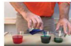
Fig. 8. Box mixing demonstration to achieve color consistency
