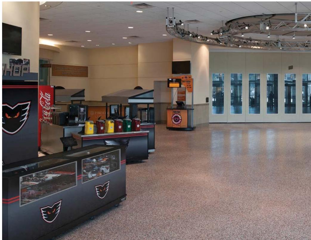
morning the Bazella Group scraped off the excess flakes for reuse, and cleaned and vacuumed the floor. A topcoat was then applied to give the floor a glossy appearance, and left to cure for six to eight hours.
