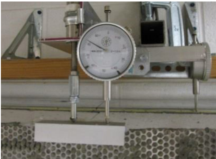
FIGURE 5 Dial Gauges to Measure Deflections
