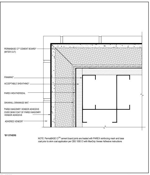
PermaBase CI cement board joints must be treated with Parex reinforcing mesh and base coat prior to skim coat application of Parex Masonry Veneer Adhesive.
