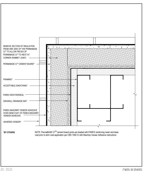
• PermaBase CI cement board joints must be treated with Parex reinforcing mesh and base coat prior to skim coat application of Parex Masonry Veneer Adhesive.
